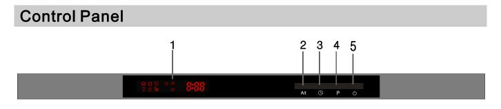
1.Display Window: To show Programs, fill rinse aid, fault codes, Dual zone wash, remaining time and delay time etc.
