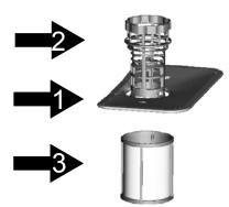
The filter system consists of a coarse filter, a flat (Main filter) And a microfilter(Fine filter).
