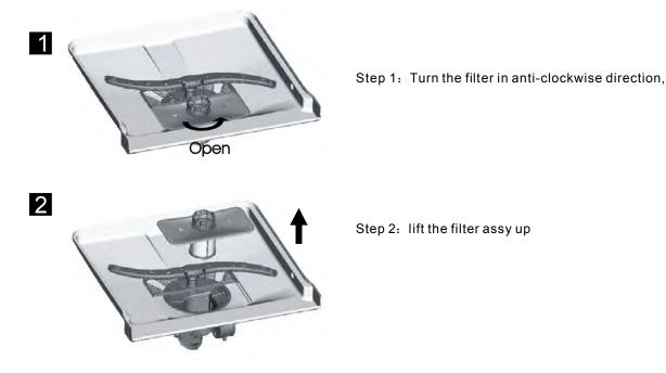
NOTE: When following this procedure from step1 to step 2, the filter system will be removed; when following it from Step 2 to Step 1, the filter system will be installed.
