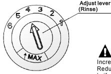
The rinse aid dispenser has six or four settings. Always start with the dispenser set on "4". If spots and poor drying are a problem, increase the amount of rinse aid dispensed by removing the dispenser lid and rotating the dial to "5". If the dishes still are not drying properly or showing spots, adjust the dial to the next higher lever until your dishes are spot-free. The recommended setting is "4". (Factory value is "4".)
