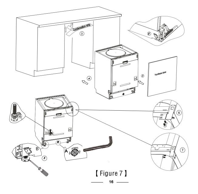
Dishwasher must be level for proper dish rack operation and wash performance.
