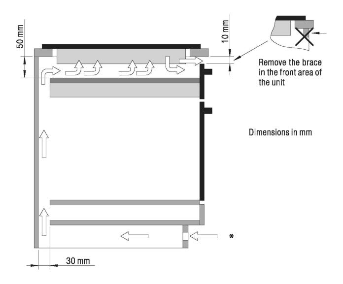
**IMPORTANT:** In the case of units with base plinths, a front grill is necessary which allows an input section of at least 100 sq. cm.
