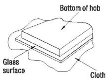
**Step 2:** Apply the strip seal, supplied with the hob, which is for sealing it onto the work surface. Do not use silicone. Apply the seal to the edge of the bottom of the hob, about 3mm from the edge of the glass. Apply the seal all around the circumference. Cut any excess and bring the two ends of the seal together so they match.
