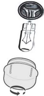
**IMPORTANT:** Replace only with a suitable 'high temperature' bulb 25W, 220-240V, T300°C.
