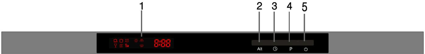
1. Display Window: To show Programs, fill rinse aid, fault codes, Dual zone wash, remaining time and delay time etc.
