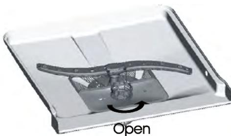
Step 1: Turn the filter in anti-clockwise direction,
